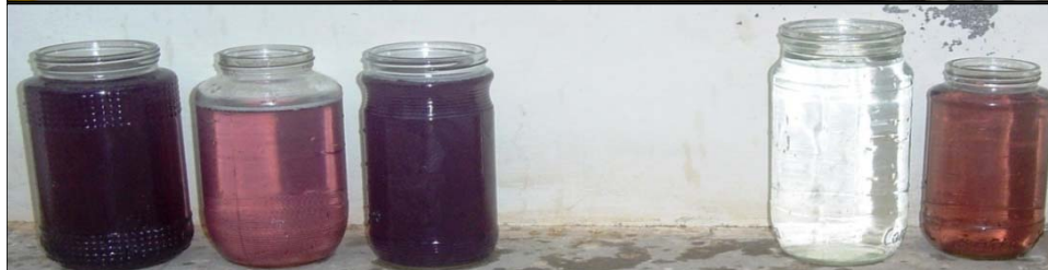
UF Feed Permeate Backflush RO Permeate Reject
