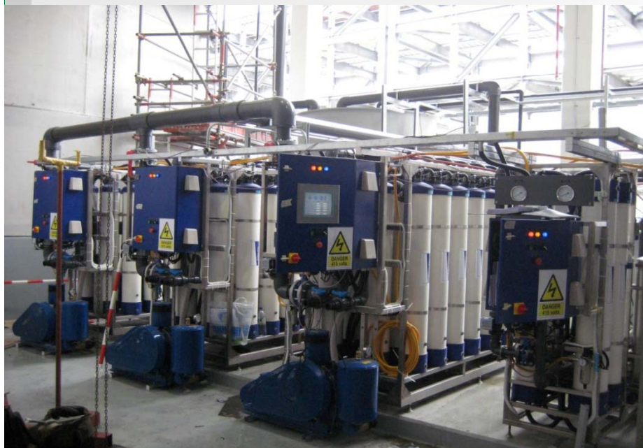
3 x MU36-8 were used to clarify 2,000 m 3 /day of wafer sawing water with high COD.
