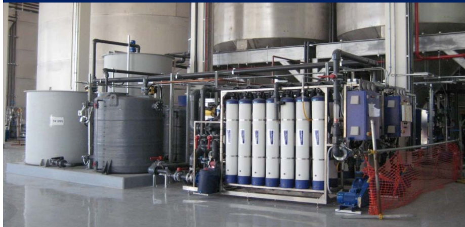
3 x MU36-8 were used to clarify 2,000 m 3 /day of wafer sawing water with high COD.
