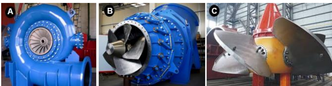
Figura 22: (a) Turbina Francis; (b) Turbina Kaplan; (c) Turbina Hélice (Adaptado Mecânica Industrial, 2017)
